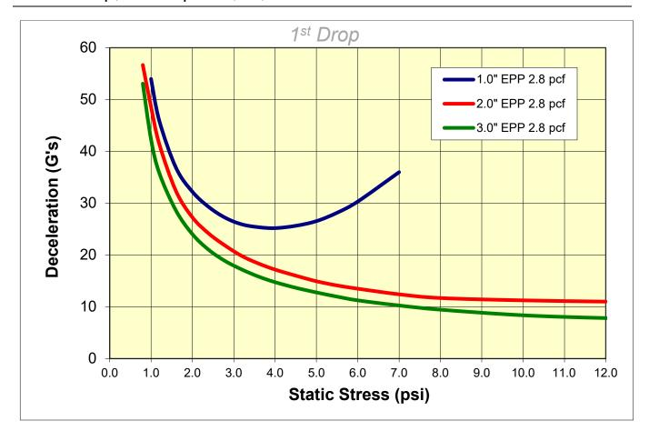
Notes: 45 g/l = 2.8 pcf = 20 X (g/l = grams per liter; pcf = pounds per cubic foot; X = foam expansion ratio) Reference: ASTM D1596; Tested at ambient conditions
