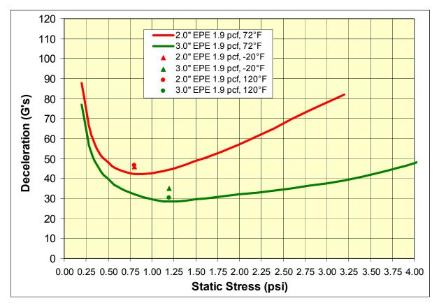
Note: 1.9 pcf = 30 g/l = 31X (g/l = grams per liter; pcf = pounds per cubic foot; X = foam expansion ratio) Hot and Cold Drop/Impact performed at Peak (MIN) G-force for given thickness.
