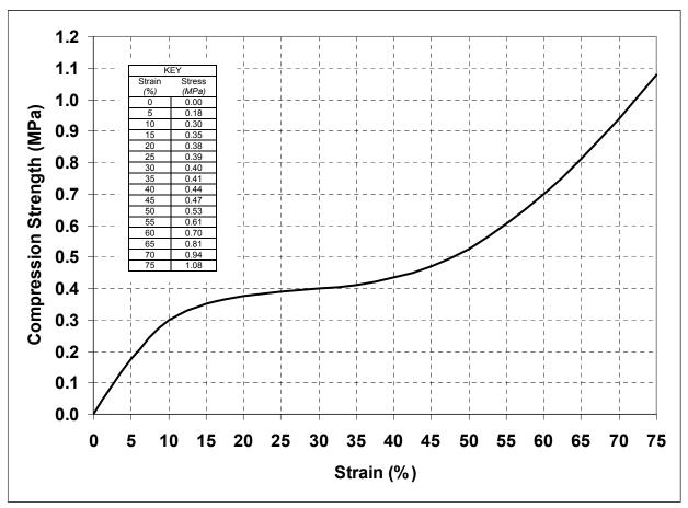
Note: 60 g/l = 3.75 pcf = 15 X (g/l = grams per liter; pcf = pounds per cubic foot; X = foam expansion ratio) 1 MPa = 1 N/mm<sup>2</sup> = 145.04 psi (Units of pressure/stress) Test Speed at 12.5 mm/minute (per ASTM-D3575)
