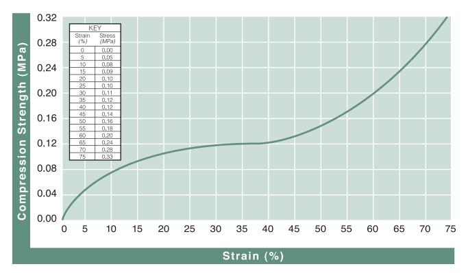
Note: 20 g/l = 1.25 pcf = 45X (g/l = grams per liter; pcf = pounds per cubic foot; X = foam expansion ratio) 1 MPa = 1 N/mm<sup>2</sup> = 145.04 psi (Units of pressure/stress) Test Speed at 12.5 mm/minute (per ASTM-D3575)
