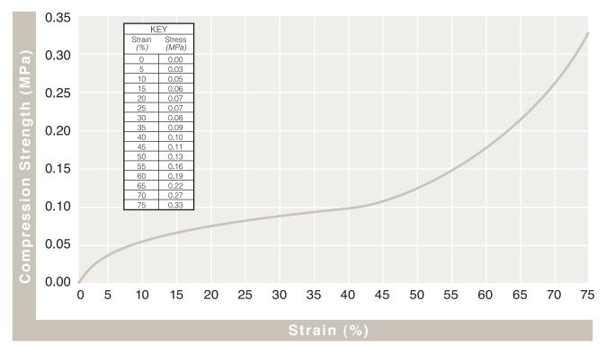
Note: 24 g/l = 1.5 pcf = 37 X (g/l = grams per liter; pcf = pounds per cubic foot; X = foam expansion ratio)  $1 \text{ MPa} = 1 \text{ N/mm}^2 = 145.04 \text{ psi (Units of pressure/stress)}$ Test Speed at 12.5 mm/minute (per ASTM-D3575)
